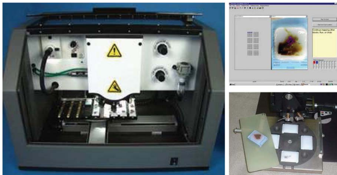
Fig. 1. ATA-27 automated arrayer.
