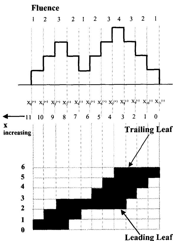
Fig. 5. Ma's algorithm for MLC leaf sequence (Ref 9)
