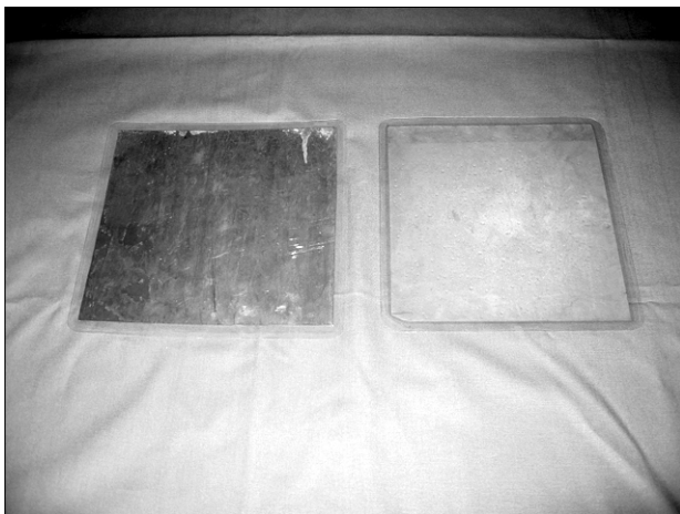
Fig. 3. The Pb 0.5 mm thickness of filter for standard (Left) and experimental lead-free shielder (Right) which is 200 \times 200 \times 1.5 \text{ mm}^3 of size for 0.42 mm Pb equivalent.
