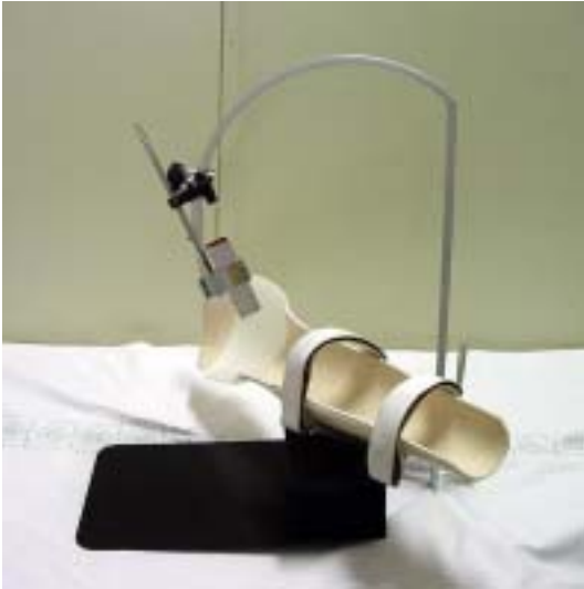
Fig. 1. Special device, which was designed for holding transducer and arm in the same position without movement.
