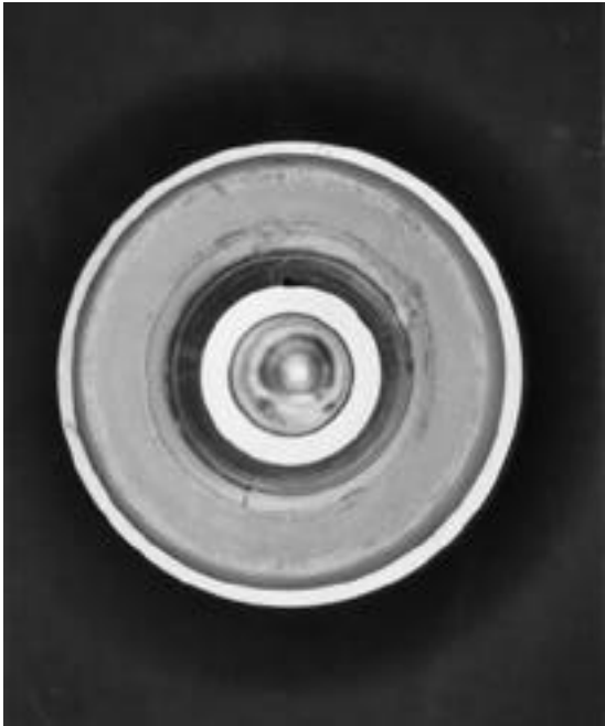
Fig. 3. Retrieved bipolar cup shows significant wear on the polyethylene rim.
