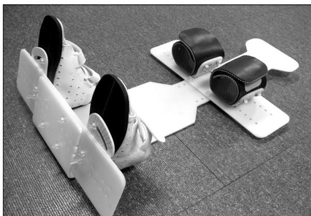
Fig. 2. A device for computed tomography of the tibia.
