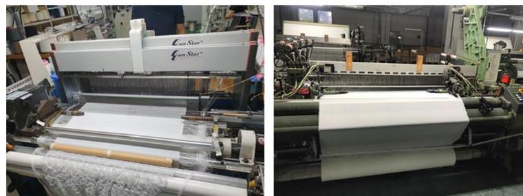
**Figure 4.** Shielding fabric weaving process conducted using an HTVS 8/S20 machine.
