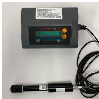
**Figure 6.** Low-dose radiation measuring equipment (Radcal 2186 [Accu-Dose], Radcal Co, 2017, Correction 2020).
