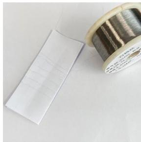
**Figure 1.** Tungsten wire (50  $\mu\text{m}$ ) used in the manufacture of the shielding fabric.
