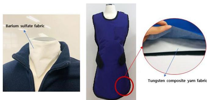
**Figure 7.** Prototype radiation shield clothing: (a) scarf made from PET containing BaSO<sub>4</sub> and (b) (with inset) apron and radiation shield clothing items manufactured using the tungsten composite fabric.
