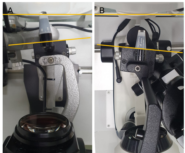
Figure 5. Applanation tonometers mounted along monocular axis of stereo-microscope. (A) Goldman tonometer model 900.4.4 on Haag-Streit slit lamp is examined through the right eyepiece of the stereo-microscope. The axis is slightly rotated counter-clockwise. (B) Goldman tonometer model 900.4.2 on Huvitz slit lamp is examined through the left eyepiece of the stereo-microscope. The axis is slightly rotated clockwise.
