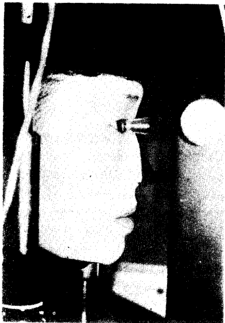
Fig. 3. Transducer with frequency of 15MHz.
