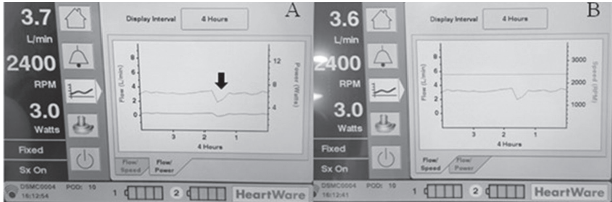
Fig. 2. HeartWare™ monitor parameters during operation. (A) both Power (Watts) and Flow (L/min) decreased soon after the induction of anesthesia (black arrow). (B) Speed (RPM) was constant throughout the operation.
