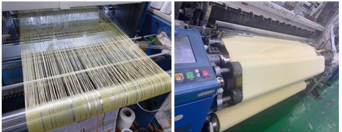
**Figure 3.** Para-aramid double-weave fabric weaving process.
