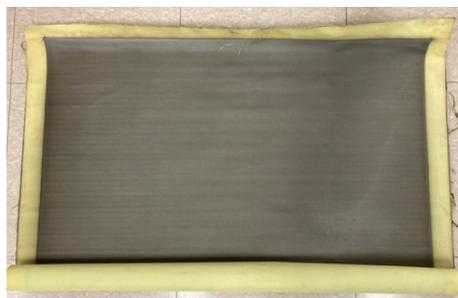
**Figure 11.** Finished tungsten-coated shielding fabric.
