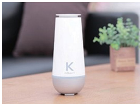
Fig. 2 AirguardK® (Kweather, Co, Korea); a device for measurement of air pollutants, placed inside the participants’ house at least 1 week per trimester
