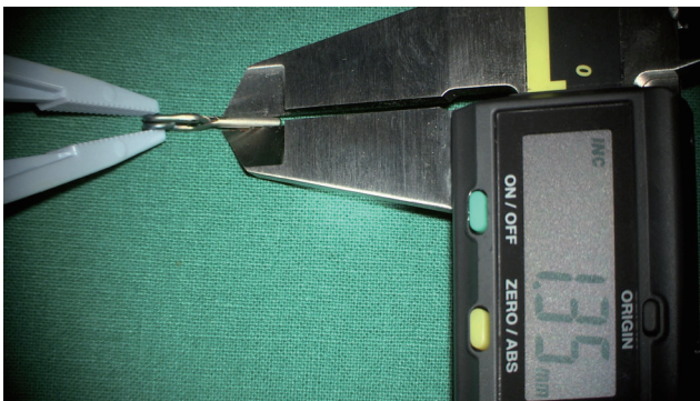
Fig. 3. Digital precision ruler to measure the thickness of the aneurysm clip blade.
